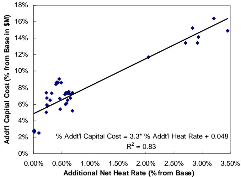
**Figure 3.4** Relationship between Heat Rate and Capital Cost for Environmental Controls on a PC Plant (Source: IECM, 2004)
