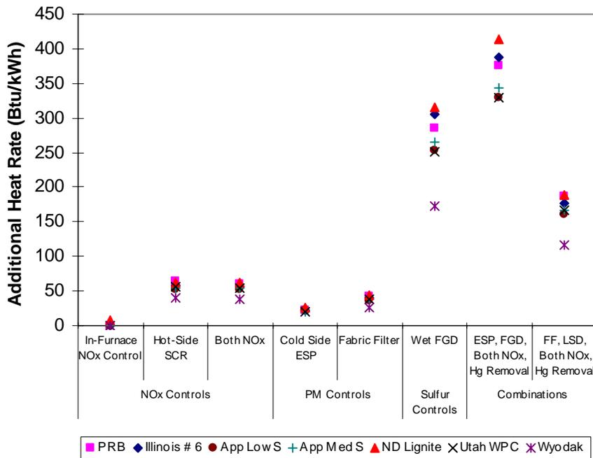
**Figure 3.3** Efficiency Penalties of Environmental Control Technologies for a Subcritical Pulverized Coal Plant (Source: IECM, 2004)
