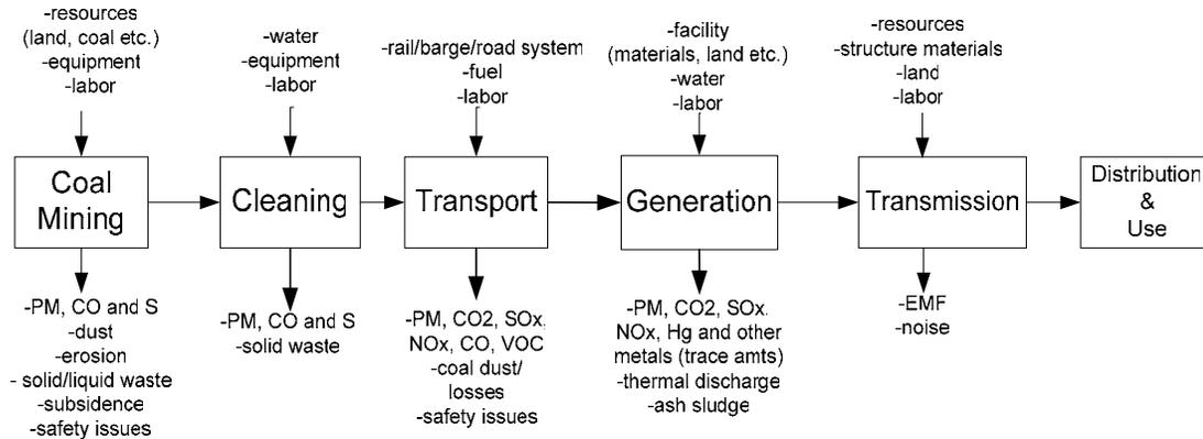
**Figure 3.1** Simplified Life Cycle of Coal-Fired Electricity.
