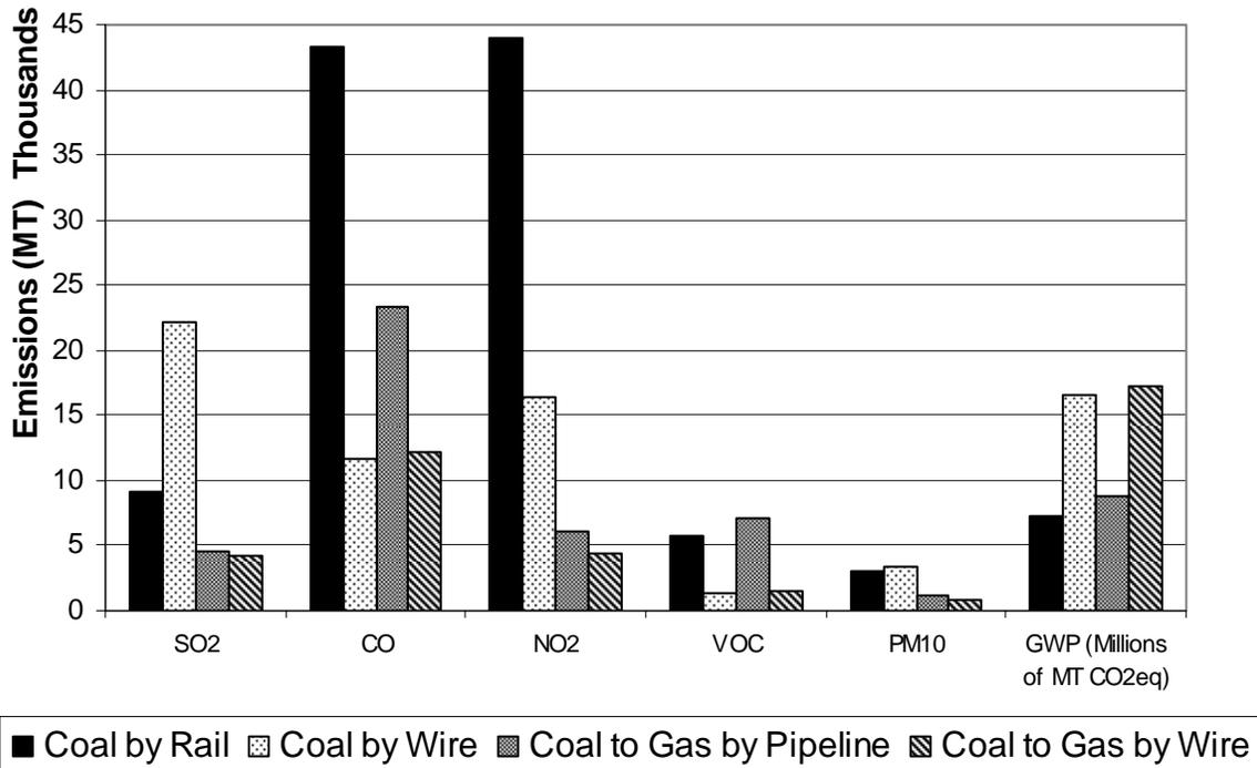
**Figure 4.2** Comparison of Emissions for the Four Methods of Transporting Energy from the PRB to Dallas Over 30 Years.
