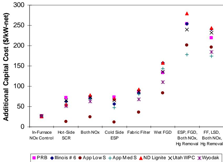
**Figure 3.2** Cost Penalties of Environmental Control Technologies for a Subcritical Pulverized Coal Plant (Source: IECM, 2004)
