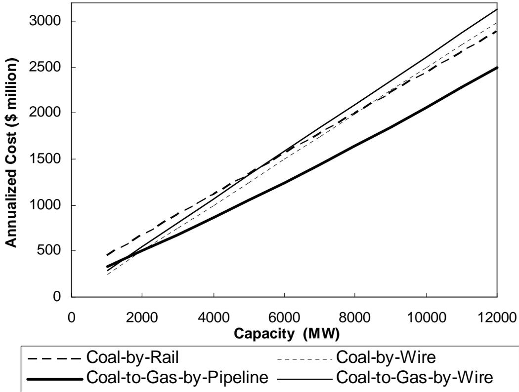
**Figure 4.3** Annualized System Costs with Varying Amounts of Electricity Delivered
