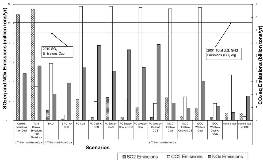
**Figure 5.4** Annual Life Cycle Emissions (SO<sub>2</sub>, CO<sub>2</sub>, and NO<sub>x</sub>) for Coal and Natural Gas Scenarios.
