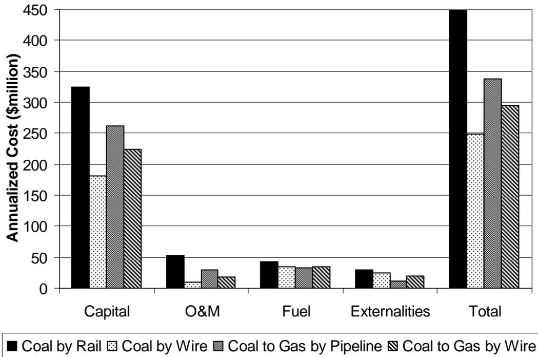
**Figure 4.1** Summary of the Cost for Four Methods of Transporting Energy from the PRB to Dallas Assuming New Infrastructure Required for Each Option in the Base Case.
