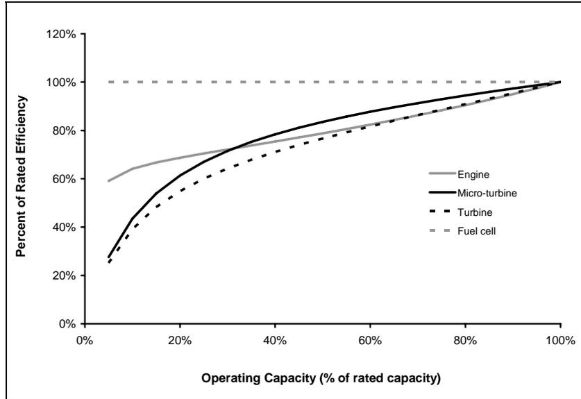
**Figure A-5.** Partial-load efficiency curves. When an engine, micro-turbine, or turbine is operated at less than its rated capacity, it operates with less efficiency. Fuel cells do not exhibit this behavior. The partial load efficiency curves vary by technology, and are defined by quadratic functions.
