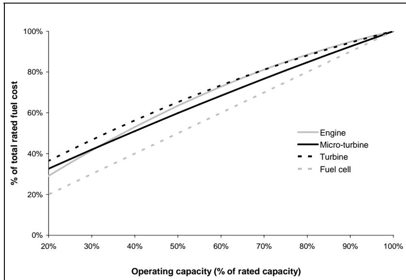
**Figure A-6.** Fuel cost curves. When an engine, micro-turbine, or turbine is operated at less than rated capacity, it operates less efficiently and consumes proportionately more fuel. The fuel cost curves vary for each technology, and are defined by quadratic functions.
