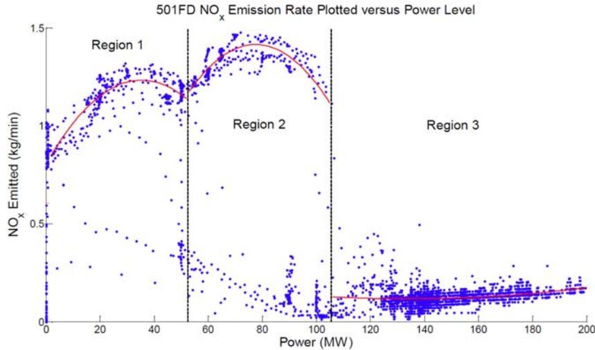
Figure 4.  $NO_x$  emission data from a 501FD gas turbine as a function of power (blue dots).<sup>33</sup>
