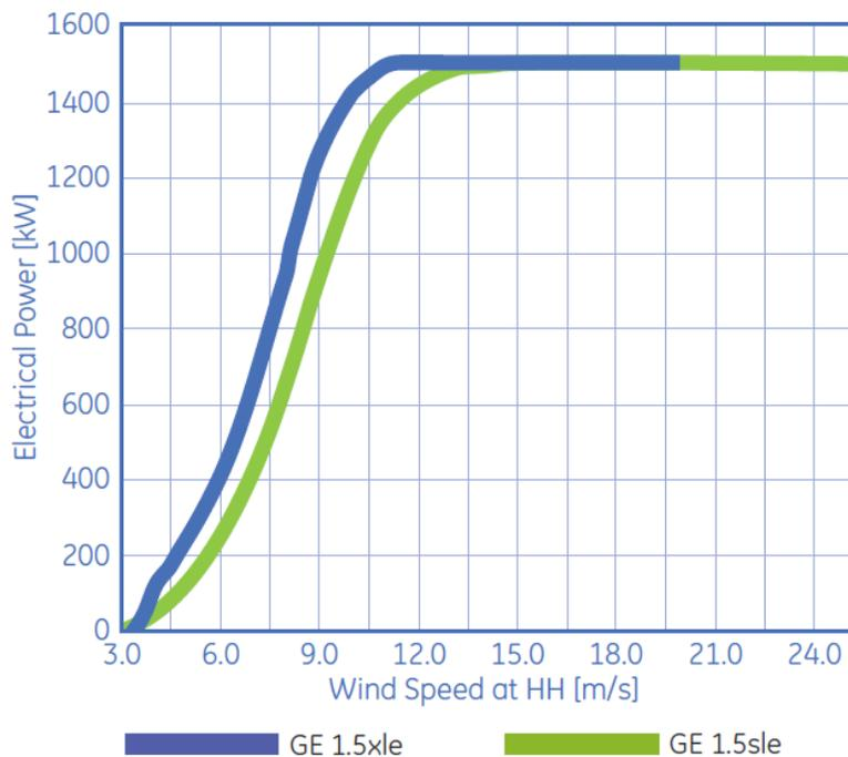
Figure 3. Electrical power output as a function of wind speed at hub height (HH) for a GE 1.5MW turbine.<sup>29</sup>
